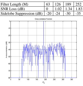
Figure 4 ACF of N=63, PSO (Mismatched Filter length M= 189) mismatch loss = 1.34db
