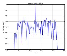
Figure 3 ACF of N=63, PSO (Mismatched Filter length M=126) mismatch loss=1.02db Table 1: Results obtained for length 63,126,189,252
