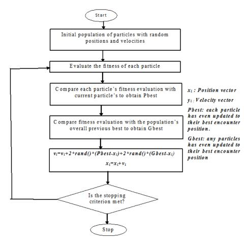
Figure 1: Working of PSO Algorithm
