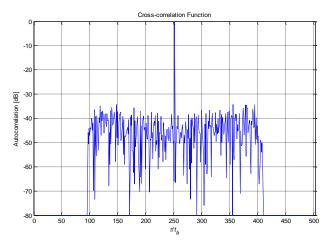
Figure 5 ACF of N=63, PSO (Mismatched Filter length M= 252) mismatch loss = 1.83db
